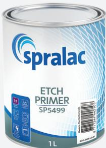
The EU VOC compliant SP5499 Etch Primer is developed with etching properties to isolate and protect old, cured coatings, steel, galvanized steel and most types of aluminium from corrosion. This beige coloured primer has a 1:1 mixing ratio with a dedicated hardener and is air dry in only 10 minutes.
